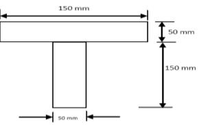
b) Determine of moment of inertia of rectangular section about the x-x axis and about the y-y axis passing through the C.G.
